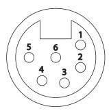
The front panel MIDI connector is a female 6-pin XLR connector. This connector carries MIDI data in both directions as well as phantom power. This connector is wired in parallel with the rear panel MIDI input, so it is very important to only use one of the two connectors at a time.
